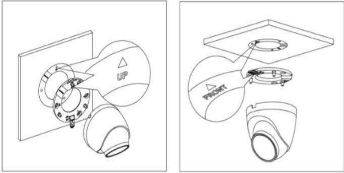
Insert the screws and using a Phillips head screwdriver, secure the installation bracket to the mounting surface.
