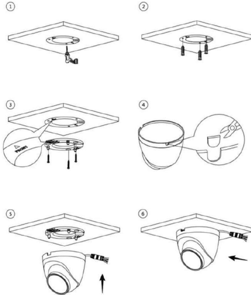
**Step 1:** Place the installation template sticker on the mounting surface. Then, using a drill, drill 3 installation holes.
