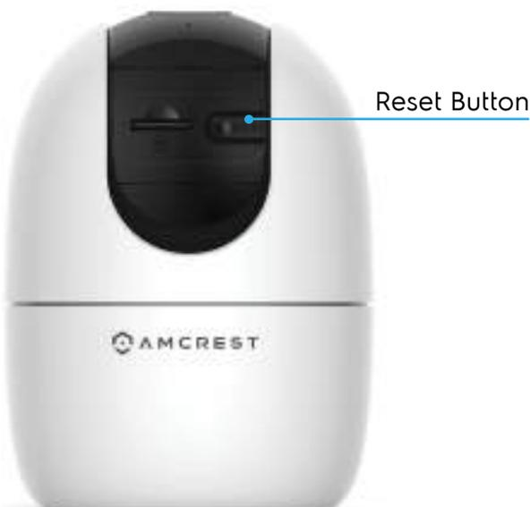
To perform a factory reset on your camera, raise the camera upward and locate the reset button.
