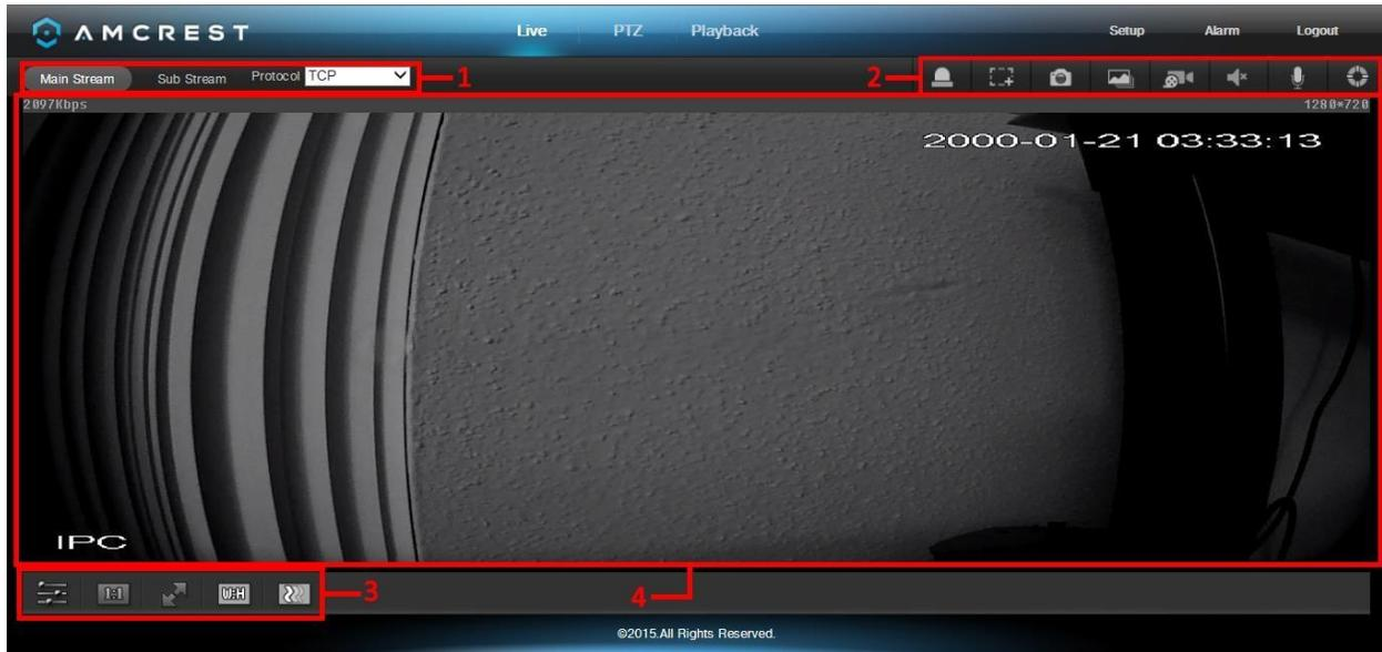
**Section 1:** This bar allows the user to select which stream type and which protocol they want to choose. For more information on stream types, see section 5.3.1.2.1. For more information on protocols, see section 5.3.2.2.1.
