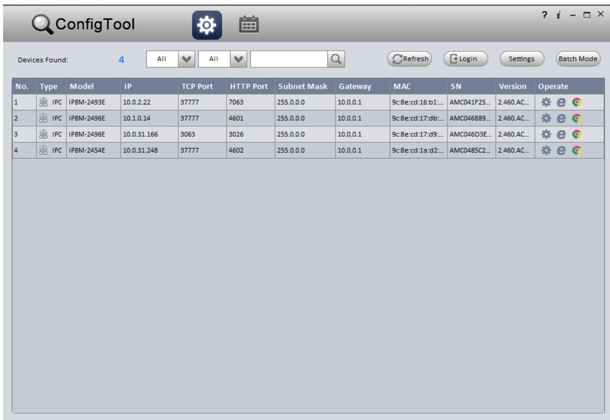
After launching the IP Config tool, click the **Refresh** button to bring up the cameras on the network.
