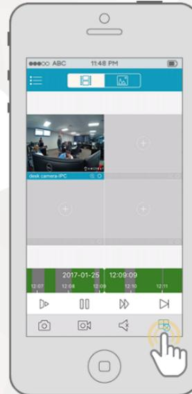
Tap the "close all windows" icon in the lower right hand corner to stop viewing recorded footage. Repeat steps 3 through 20 to view footage from additional cameras.
