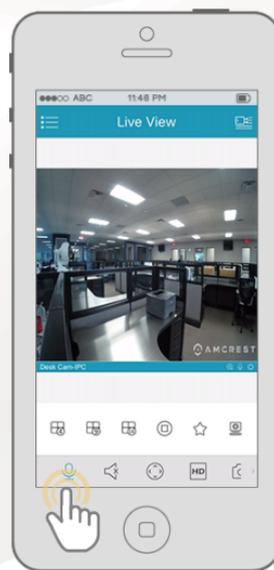
Tap the Microphone icon on the bottom left and speak once it is highlighted. Your voice will transmit to the camera for others to hear in the camera's vicinity.
