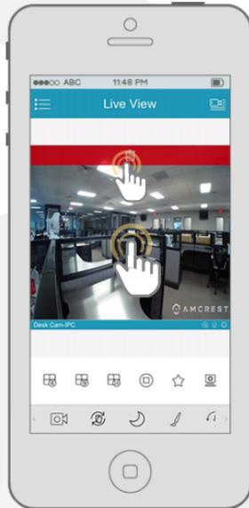
**Note:** To close a previously opened camera window, tap and hold on the video until the trash can icon is shown, then drag to the trash can icon. This removes the camera and allows you to replace it with another camera feed.
